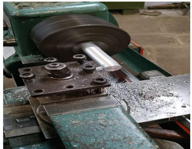
Fig -8: Machining of Specimens as per ASTM Standard
