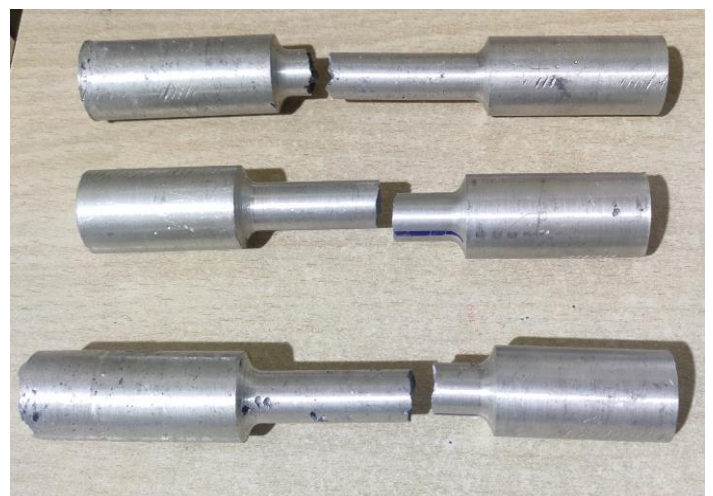
Fig -10: Test Specimens after Tensile Test
