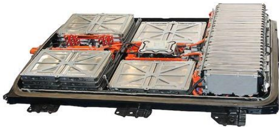
Fig -5: Battery system with individual cells in series
