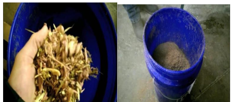
Fig.1. Collected wooden chips (left) and converted to 2mm uniform particle size (right).
