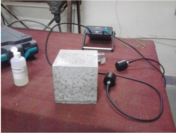
Fig. 2: UPV Test of concrete specimen
