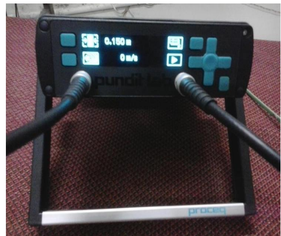
Fig 1: UPV Test apparatus
