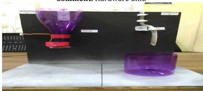
Comment: Dispenser unit for dispensing goods. First dispenser is used to dispense solid and second is used to dispense liquid.
