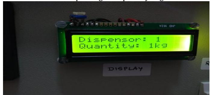
Comment: displays the dispenser number and quantity being dispensed through dispenser.
