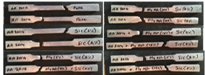
Fig 3: Work pieces before and after tensile tests
