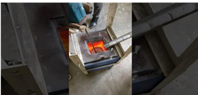
Fig 2: Stir Casting arrangement
