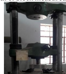
Fig-3: Flexural strength test conducted by using Universal Testing Machine
