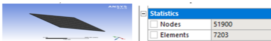
Fig 4.23 – Meshed Model of sandwich structure
