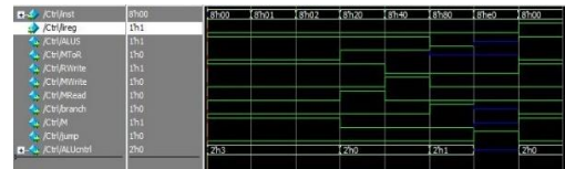
Fig4. Control unit simulation result
