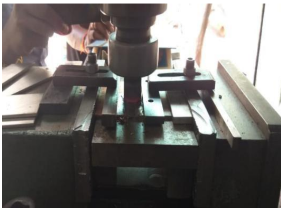
Fig: friction stir welding process
