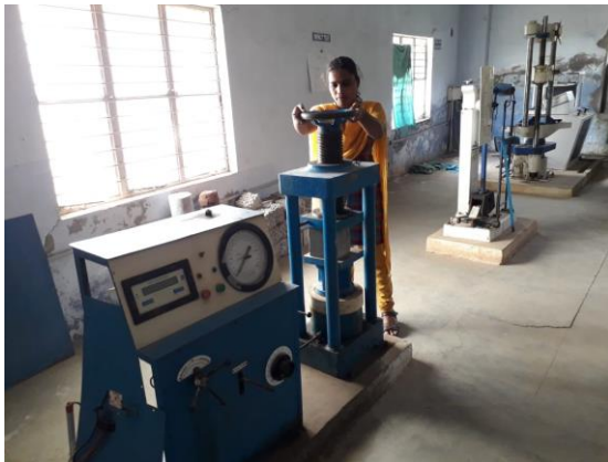
Fig.5 Compressive Strength Testing
