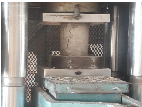
Fig 5: Concrete Cylinder is being tested for compressive strength
