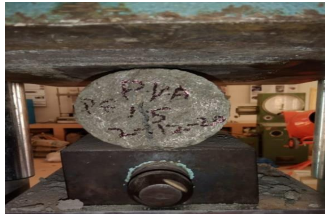
Fig 6: Concrete Cylinder is being tested for Split Tensile Strength in UTM
