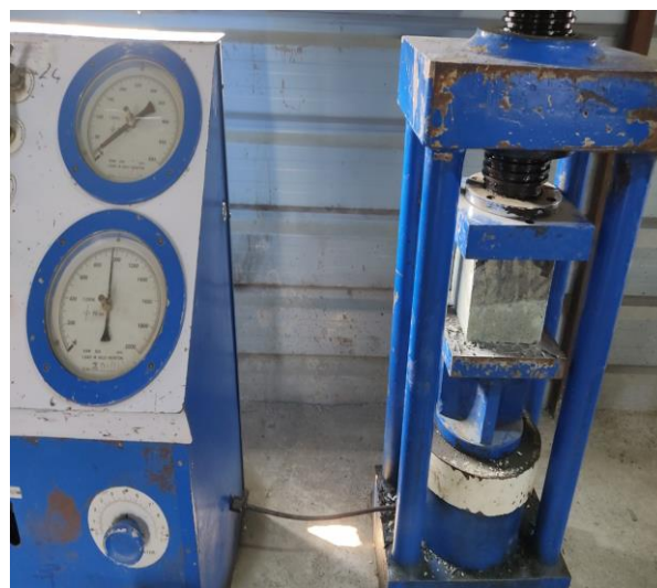
Figure 4. Compressive testing machine
