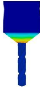
Fig 8.2 Total deformation of drill chuck
