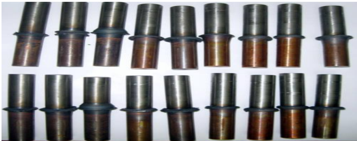
Figure 3: Specimen visual inspection of welded portion
