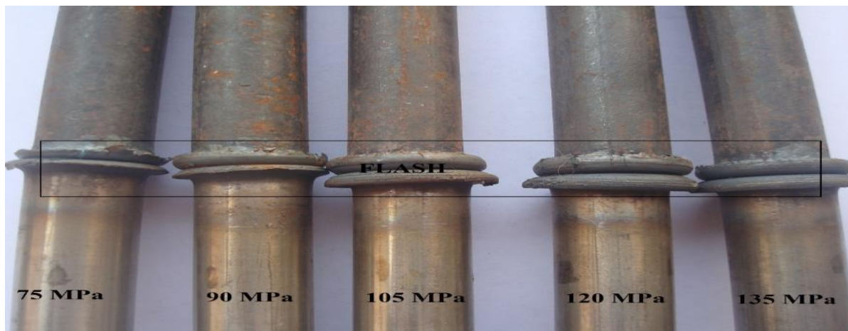
Figure 4: Specimen samples material (copper and ferritic stainless steel for friction welding at different pressure)
