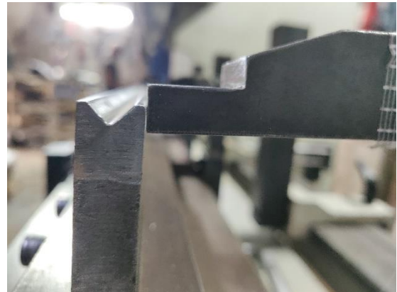
Fig-12: Collision of Stopper and Die.
