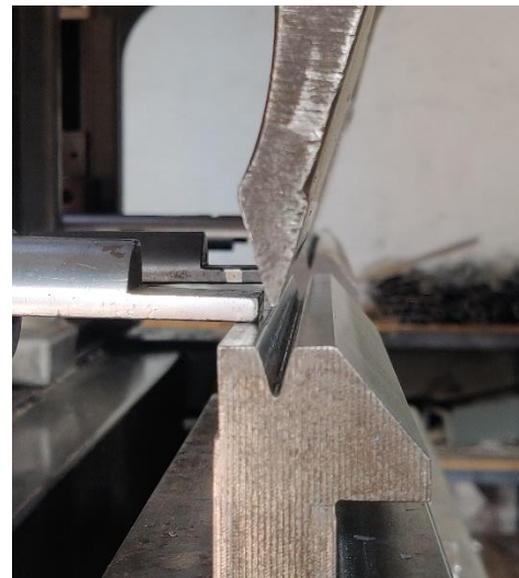
Fig-20: Actual Figure of Stopper arrangement on Die using Auxiliary Axis Adjustment Method.
