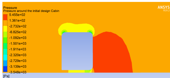
Fig - 13: Contour Plot of Pressure around the initial Cabin design
