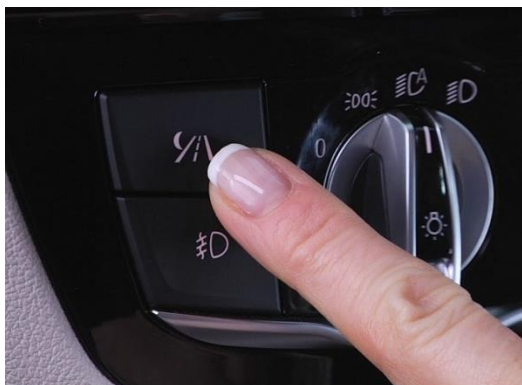
Fig -05: Button for Switch on the Night Vision used in BMW Automobiles
