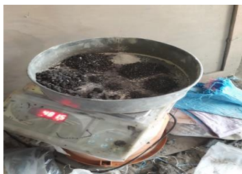
Figure-5: Weighing of aggregate
