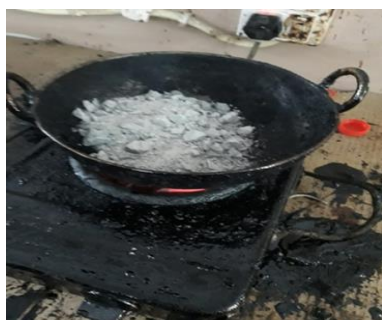
Figure-6: Heating of Aggregate & RAP mix
