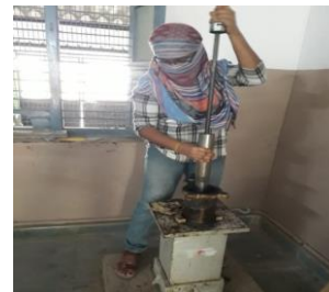
Figure-8: Compacting with 75 Blows on each side
