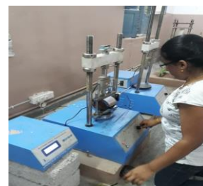
Figure-11: Testing on Marshall Test machine
