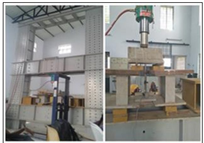
Fig-5 Roof panel testing setup
