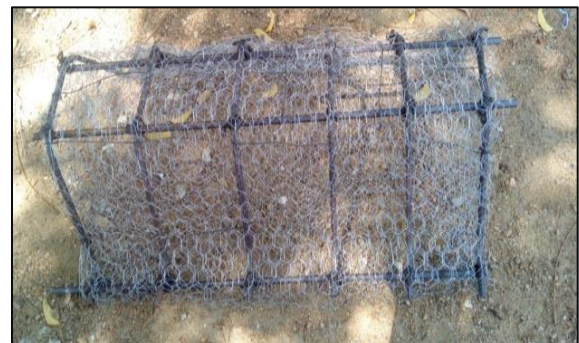
Fig- 3.3b Three layer Mesh frame
