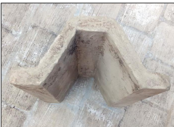
Fig-4.2a Trough shape roof specimen after casting
