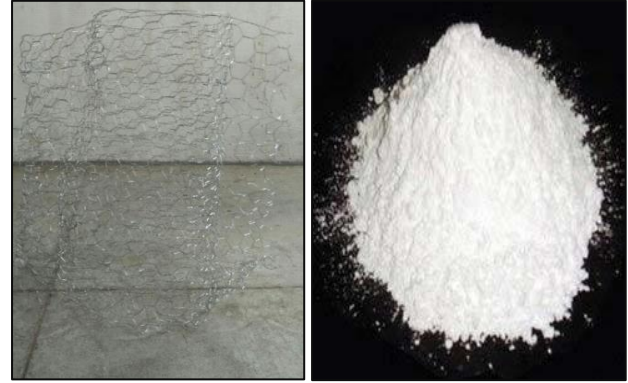
Fig-2 Wire mesh and Marble Dust Powder
