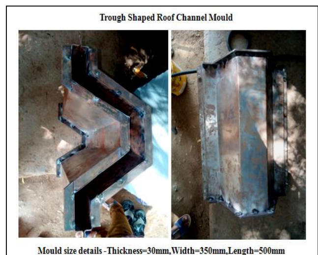
Fig-4 Trough shaped roof channel mould
