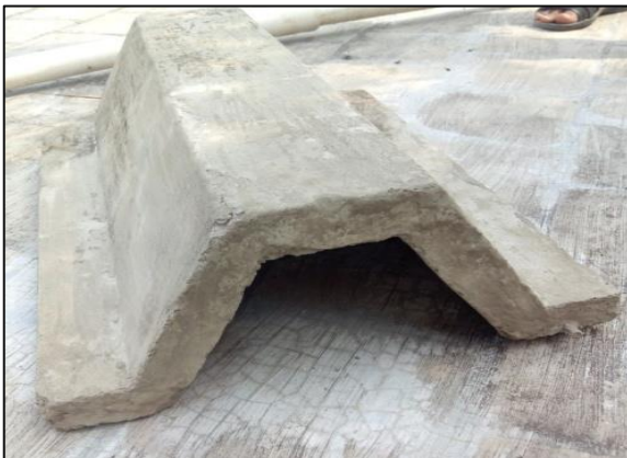
Fig-4.2 Trough shape roof specimen after casting
