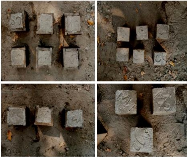
Fig-3 Casted mortar cube with MDP and without MDP
