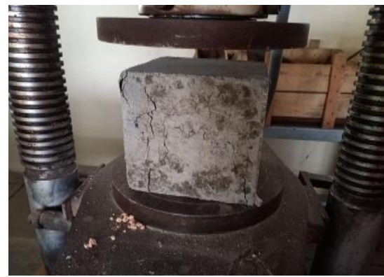
Fig 2 Compressive strength test by UTM Machine
