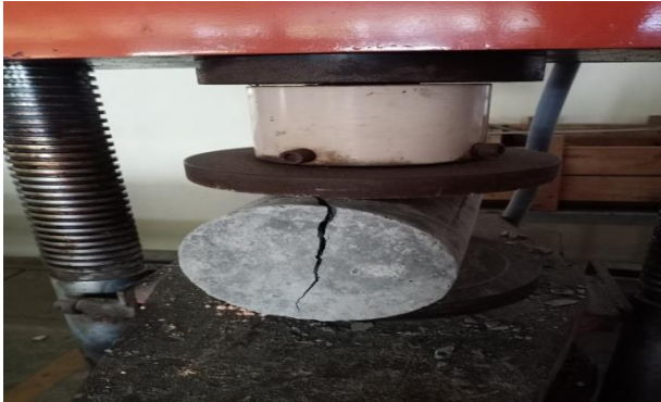
Figure 4 Split tensile strength test by UTM Machine
