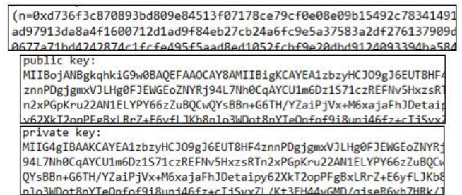
Figure 11 Sample values of a) N b) Public key c) Private key in RSA
