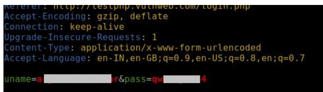
Figure 10 Sniffing credentials using Bettercap
