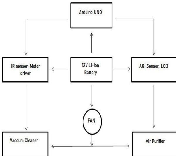
Fig.1. Block Diagram of the working of device
