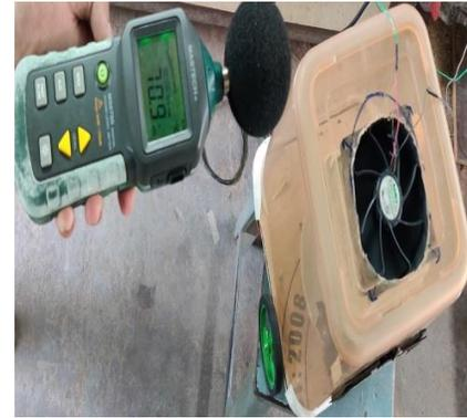
Fig.8.The result of noise level test of the device
