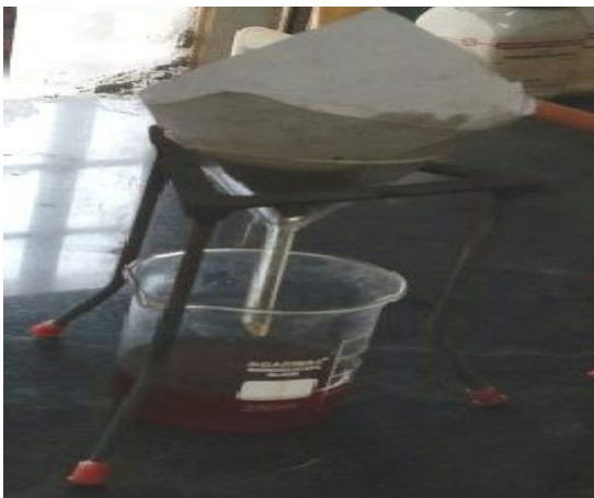
Figure 3: Filtering of oil by coffee filter
