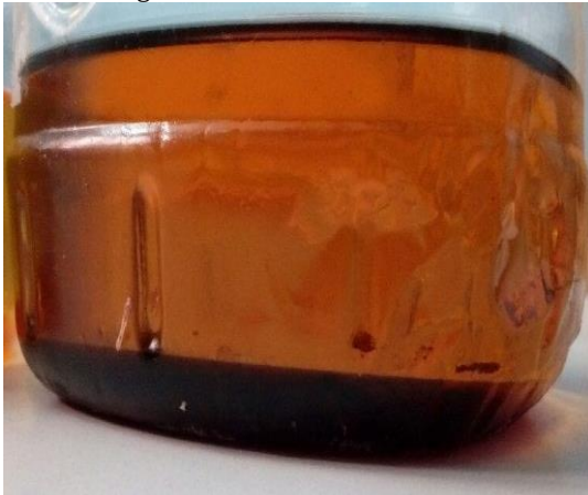
Figure 1: Separation of Heavier Impurities
