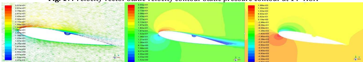
Fig. 18: Velocity vector, Static velocity contour, Static pressure contour at 15° AOA
