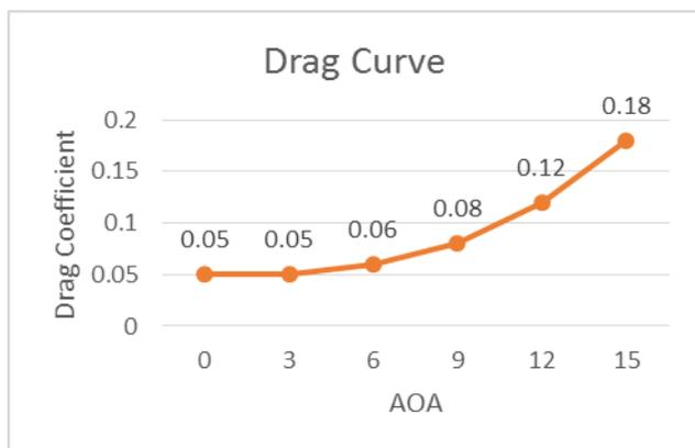
Fig 9: Drag Curve for Cropped Delta Wing
