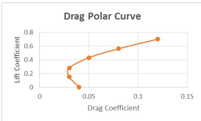
Fig 13: Drag polar Curve for Double Delta Wing
