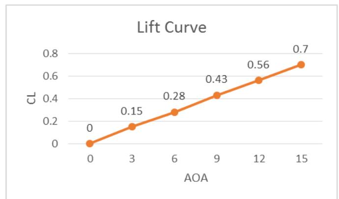
Fig 11: Lift Curve for Double Delta Wing
