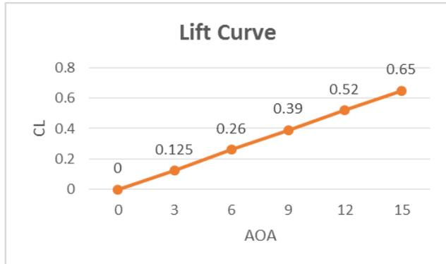
Fig 8: Lift Curve for Cropped Delta Wing
