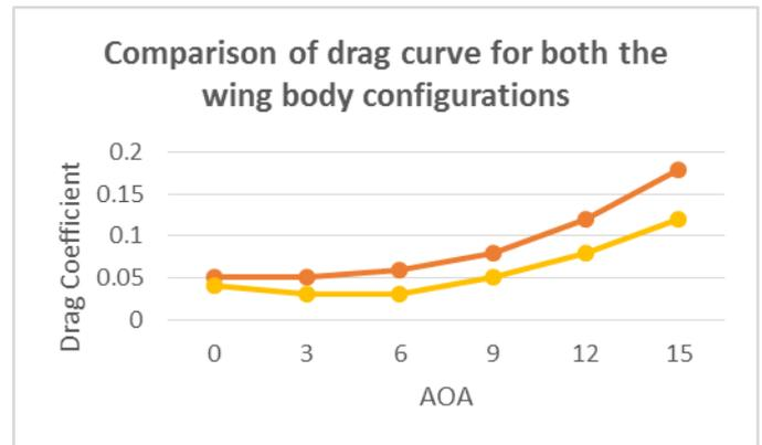
Fig 15: Drag Curve for both Delta Wing bodies
