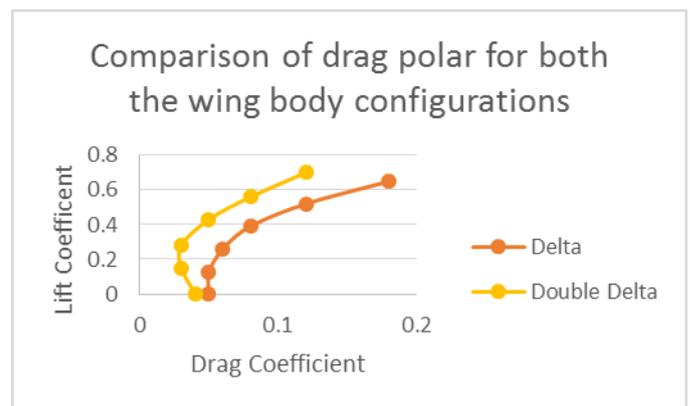
Fig 16: Drag Polar Curve for both Delta Wing Bodies
