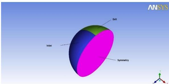
Fig 5: Segmented domain with cap
