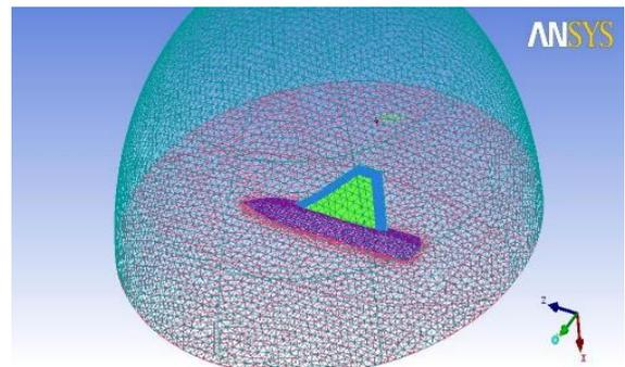
Fig 6: Meshed model of double delta wing body with domain
