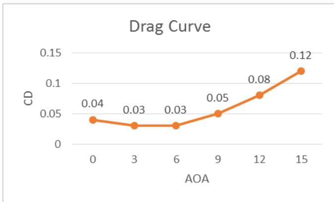
Fig 12: Drag Curve for Double Delta Wing
