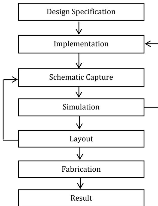
Fig -3: VLSI Design Flow Chart
