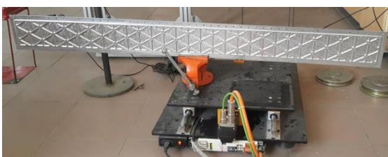
Figure -16: Free vibration test moment
