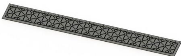
Figure -2: Isogrid aircraft lid CAD design image
