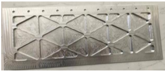
Figure -4: Isogrid structure test sample
