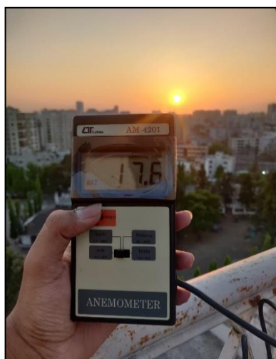
Figure 5: Reading of wind speed using Anemometer.
