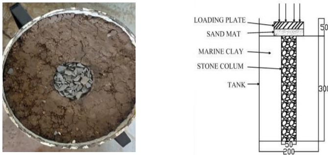
Fig-3.3.1: Clay Bed with Stone Column
