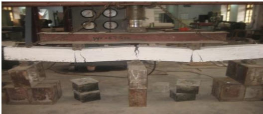
Figure 3.12 Flexural failure of CB1
