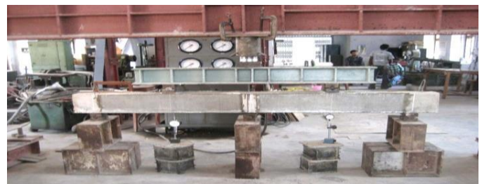
Figure 3.38 Experimental set up and strengthening pattern of TB2
