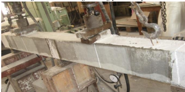
Figure 3.32 Failure of SB8 by debonding of GFRP
