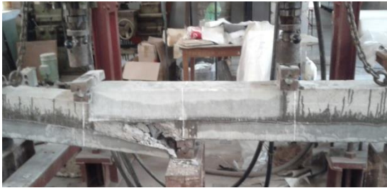
Figure 3.29 Shear crack in the left span
