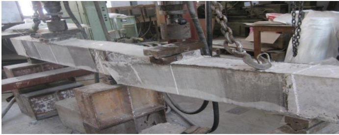
Figure 3.41 Failure of beam TB3
