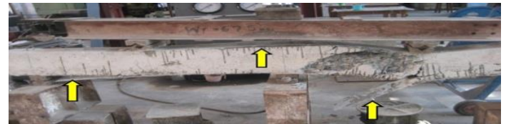
Figure 3.15 Debonding failure of FRP
