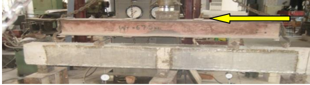
Figure 3.20 Debonding failure of FRP
