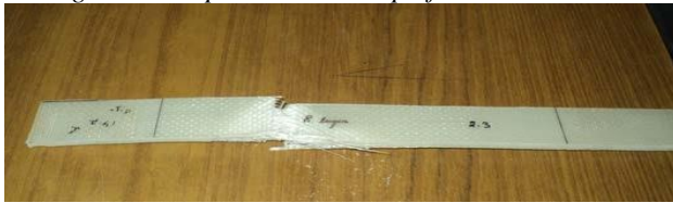
Figure 3.10 Specimen failure after tensile test
