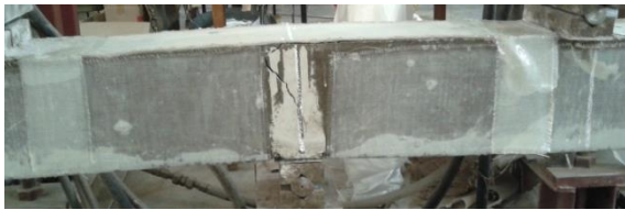
Figure 3.21 Strengthening pattern of beam SB4
