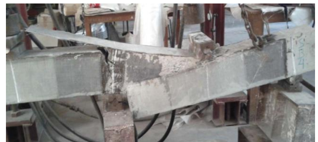
Figure 3.27 Debonding failure of Strengthened beam SB6
