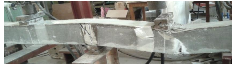
Figure 3.25 Rupture of GFRP sheet at mid section of the right span
