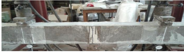
Figure 3.19 U-jacketed GFRP wrapped on the Beam SB3
