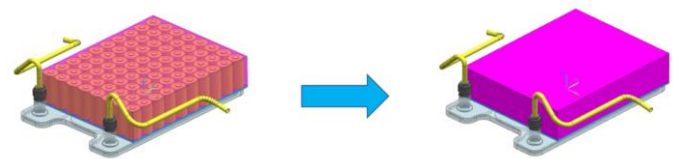
Fig -6: Representation of Battery module as Cuboid for simulation
