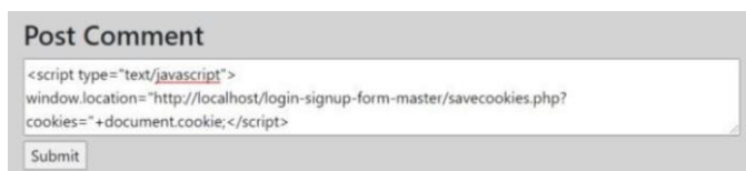
Fig - 15: Using the same JavaScript code as used in 'Fig - 9' to save the contents of the cookie in 'saved.txt' file
