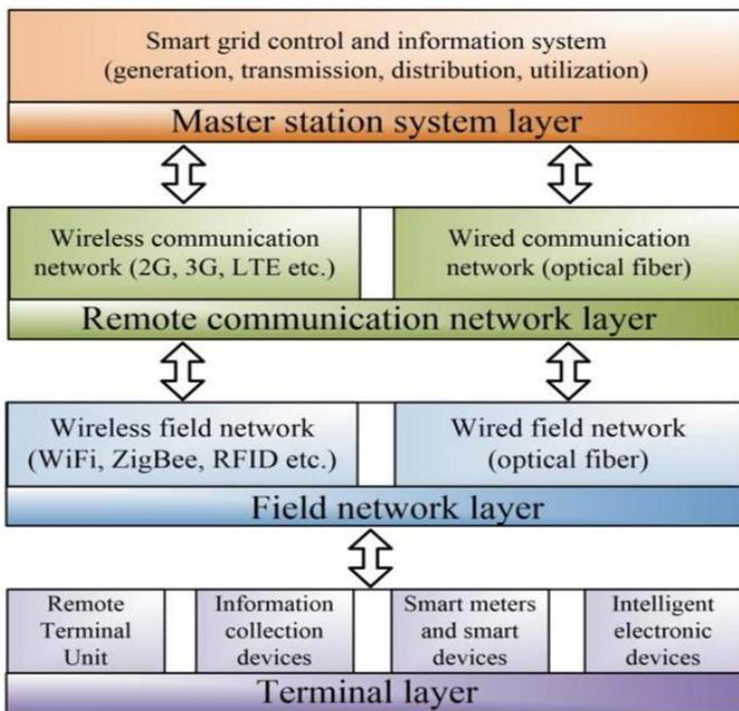
Fig -7: Four-layer architecture for IoT into SG[1]
