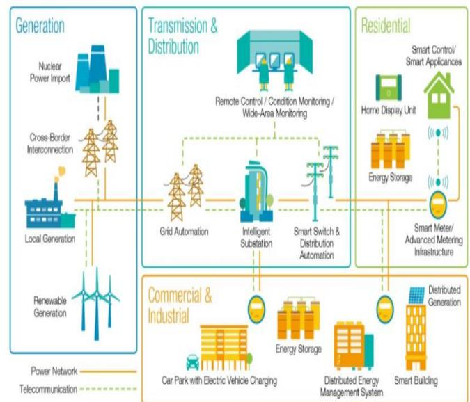
Fig -3: Integration of IoT into Smart Grid [3]
