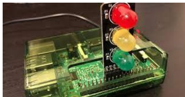
Figure 5: RASPBERRY PI 3 B+ and trafficligh LED with circuit.
