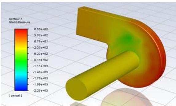
Fig -8. Pressure contour plot for blower M<sub>2</sub>
