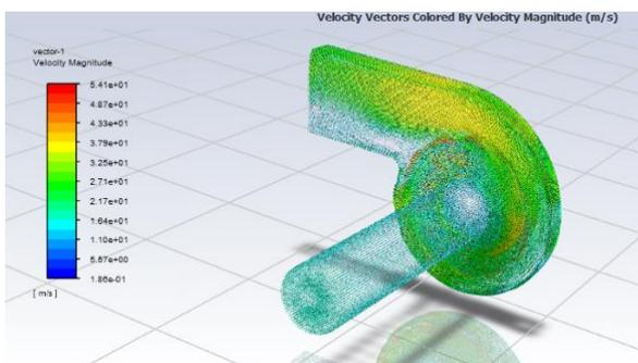
Fig -9. Velocity vector for modified blower M<sub>2</sub>
