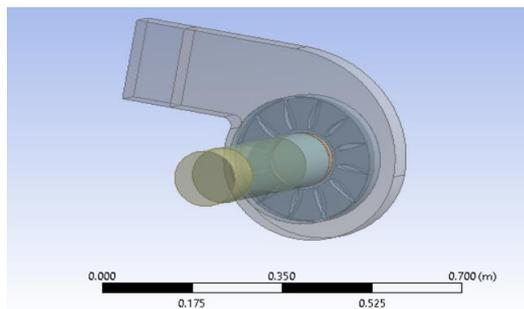
**Fig -2:** Centrifugal blower solid model with airfoil-curved impeller blades
