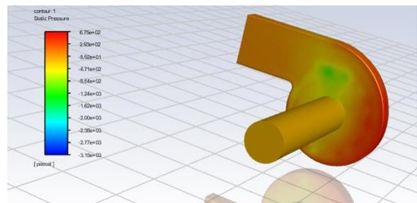
**Fig -4.** Pressure contour for blower M<sub>0</sub>
