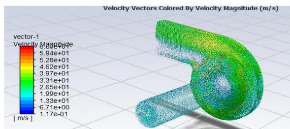
**Fig -5.** Velocity vector for blower M<sub>0</sub>
