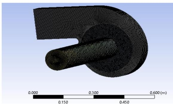
**Fig -3:** Meshing model of centrifugal blower
