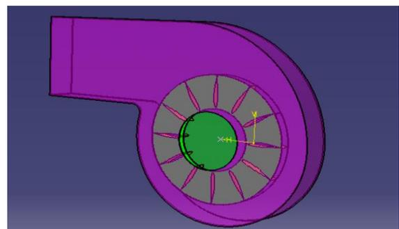
**Fig -1:** CATIA model of centrifugal blower
