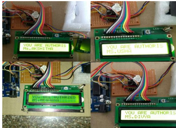
Figure 9: LCD showing the output of authorized person
