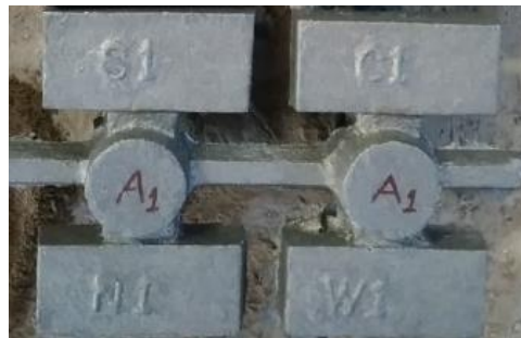
Fig. 3. Cast blocks produced using different end chills and without using chill
