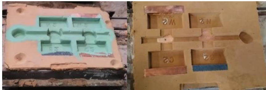
Fig. 2. (a) CO2 process sand mold and (b) Mold coated with zircon fluid
