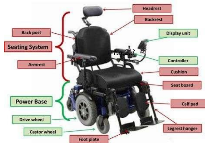
Fig.1.1: Components of Motorised Wheelchair
