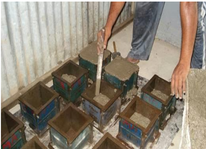
Fig -1: Cube casting in Moulds
