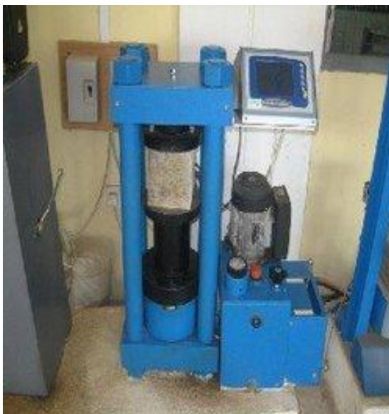
Fig -2: Testing of Cube in CTM
