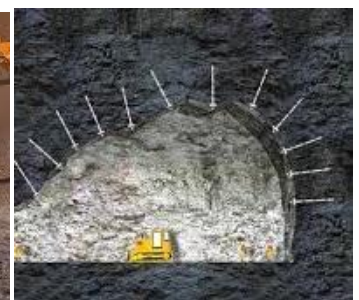
Fig -10: Rock Bolting
