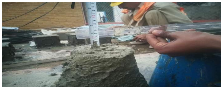
Slump Test in Lab
