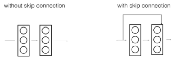
Figure 1(left) shows the working of deep Networks and (right) shows how residual network works.
