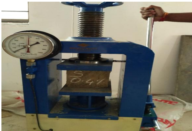
Fig4- Experimental Setup for Compression Test
