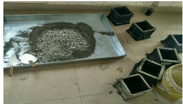
Fig 2- Hand Mixing of Concrete
