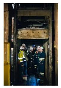
or fully enclosed models with a choice of sliding, folding, or rollup doors. Cages are used in either vertical or incline mine shafts. All cages are required to contain necessary safety features. The cage acts as transport for workers, equipment, and supplies. The unit itself is connected by steel wire rope to a hoist and, together, they function much like an elevator in a tall building.
