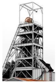
angle, with the rope positioned over the shaft by a headsheave. Shaft mining or shaft sinking is excavating a vertical or near-vertical tunnel from the top down, where there is initially no access to the bottom.
