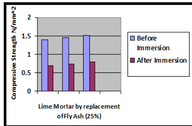
Graph10: Compressive Strength of lime mortar and replaced fly ash (25%) immersed in sulphuric acid
