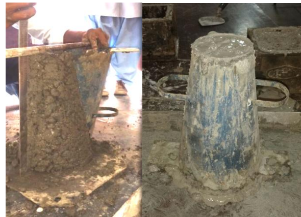
Fig -1: Slump Test
