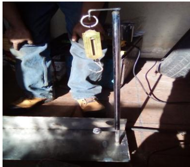
Figure 19. Dynamometer to measure string tension.
