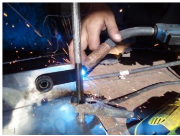
Figure 18. Welding of the pulley to the tube.
