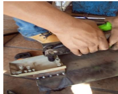
Figure 16. Tapping for motor base
