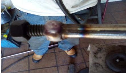
Figure 10. Pipe welded screw.
