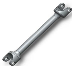
Fig- 3: CAD Model of Unibody Hollow Driveshaft with 32 mm Diameter
