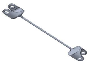
Fig- 4: CAD Model of Unibody Solid Driveshaft with 8 mm Diameter
