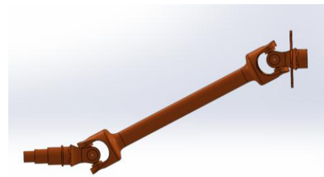
Fig- 5: Assembly of Shaft with Flange and Spindle
