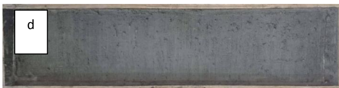
d) Surface prepared with steel brush in the transverse direction (Brush-TD)
