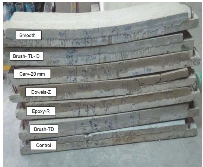
Fig. 16: Crack pattern and failure mode of the tested slabs
