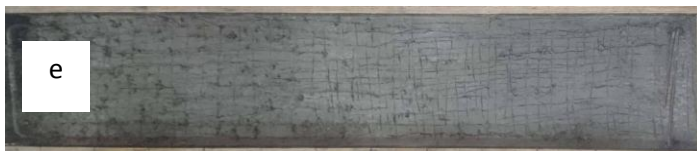
e) Surface prepared with steel brush in both the longitudinal and transverse directions (Brush-TL-D)
